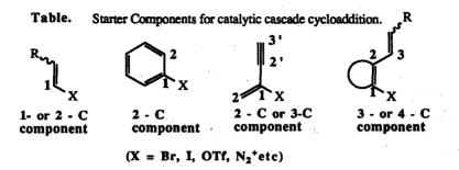
[3+2] - Processes. The aryl starter molecule (1) (5:1 E/Z isomer mixture) reacts (anisole, 120°C, 18h) with diphenyl acetylene using catalyst system  $A^3$  to give the fulvene (3) (80%) as a 5:1 Z/E isomer mixture via the vinylpalladium(II) intermediate (2).
